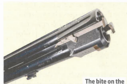
The bite on the barrel lumps can be replaced when worn
