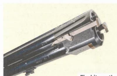
The bite on the barrel lumps can be replaced when worn
